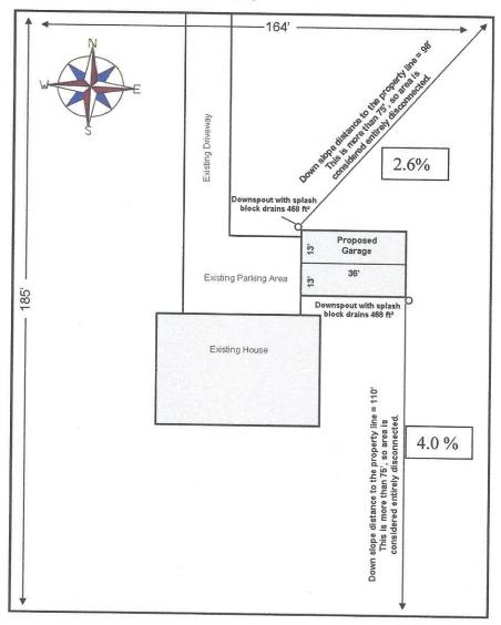
**Step 1:** Determine the area to each disconnected discharge. The area draining to each downspout is 468 ft². This is less than 500 ft², proceed to step 2.
